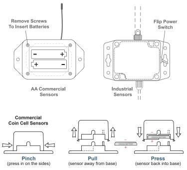
The sensor will power on within 10-20 seconds. Once online, your sensor is ready to be deployed. If you wish to change a sensor configuration, change the parameter in the software. The new parameters will be transmitted to the sensor on the next heartbeat. If you need a more immediate response from the sensor, power cycle the sensor by removing, then re-inserting the batteries or using the power switch to cycle the power.
