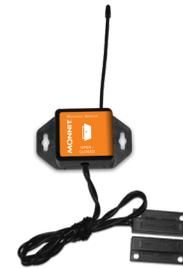
Install a coin cell battery by first taking the sensor and pinching the sides of the enclosure. Gently pull up the enclosure, separating the sensor from its base. Then slide a new CR2032 coin cell battery with the positive side facing toward the base. Press the enclosure back together; you'll hear a small click.
