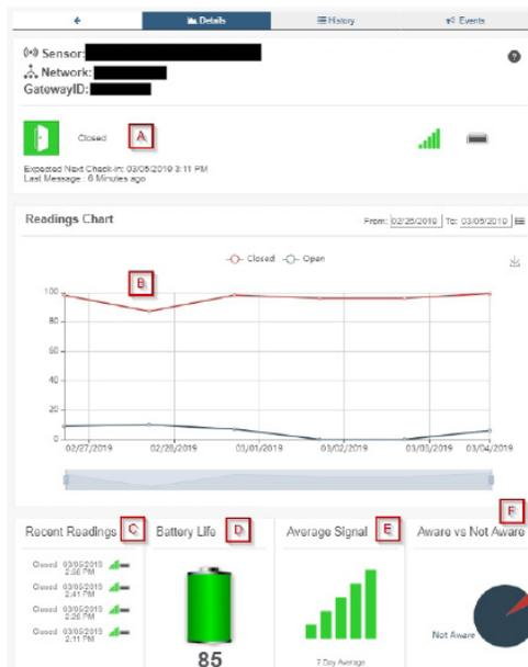
**A.** The sensor overview section will be above every page. This will consistently display the present reading, signal strength, battery level, and status.
