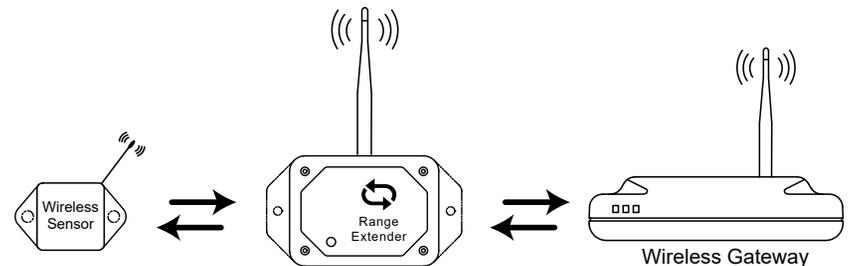
If the sensor detects a stronger signal from the range extender, it will automatically connect to the range extender.
