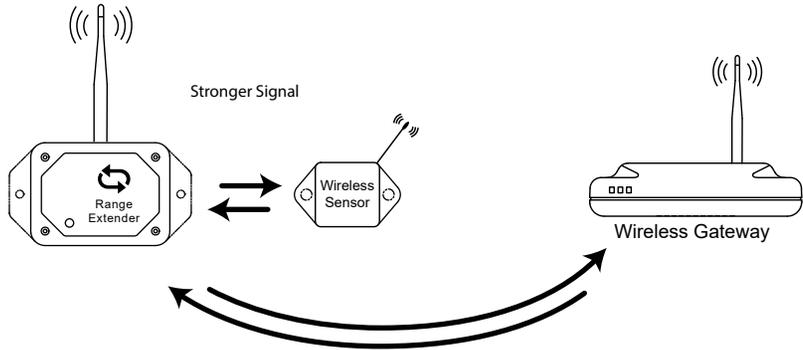
If the sensor detects a stronger signal from the gateway, it will automatically connect to the gateway and ignore the range extender.
