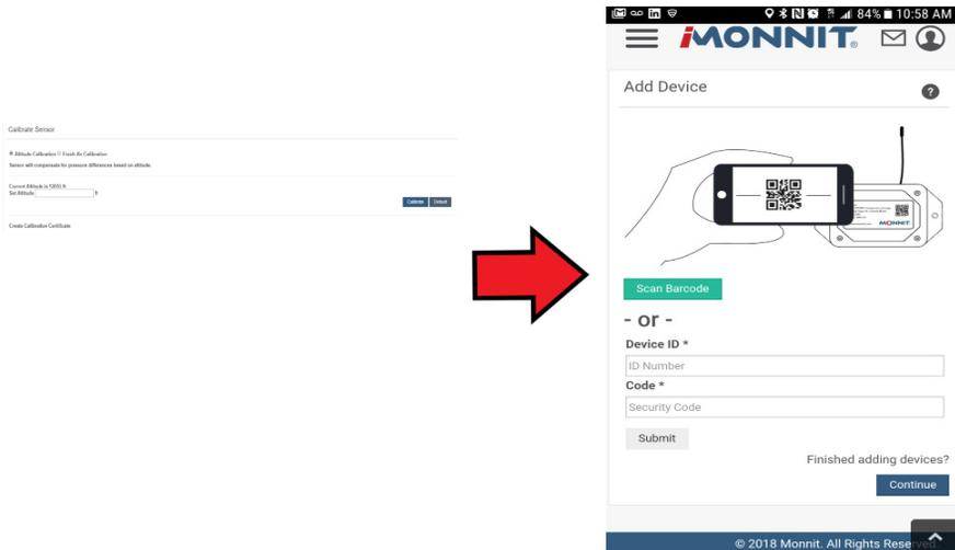
Once the range extender has been added to your network, you will need to update and push the sensor device list to your range extender so it knows what sensors to allow communication with. For a USB gateway, go to the Monnit gateway application/service and click "Download Sensor Updates". For an Ethernet gateway, power cycle the device by unplugging it, waiting 10 seconds then plugging it back in. For a Cellular gateway, use the power button to turn it off, wait 10 seconds then turn it back on.
