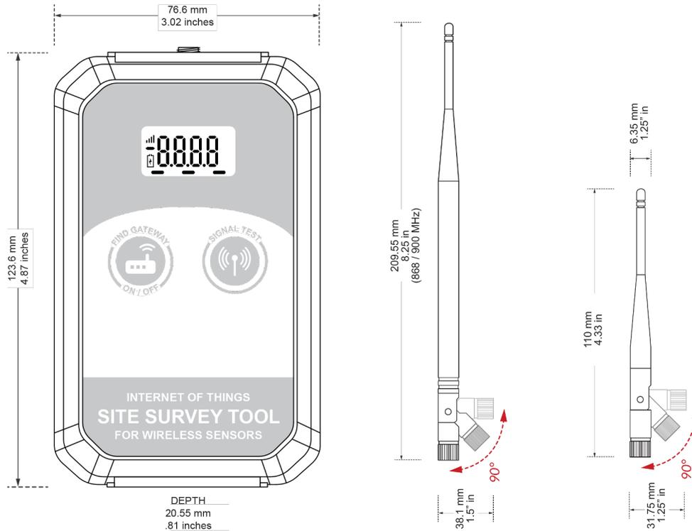
The *larger* articulated antenna is a dipole configuration and emulates the behavior of our industrial sensors with their external antenna. If you plan to buy and install **ALTA industrial sensors**, connect the dipole antenna to the ALTA Site Survey Tool.
