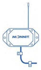
Mount the sensor. Secure the lead, if applicable.
