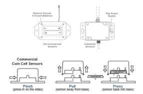
**Note**: It will take 10 - 20 seconds for the sensor to power up. Configurations for your sensors can be changed in iMonnit. Your new modifications will take effect on the next heartbeat. More immediate results can be achieved by power cycling the sensor. Power cycling is accomplished by removing then re-inserting batteries or using the power switch to cycle the power.
