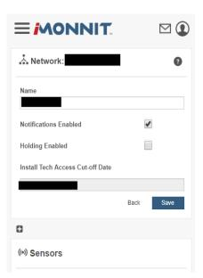
The network edit page will give the option of changing the name of your network, enable notifications, enable holding, and review the Install Tech Access Cut-off Date.
