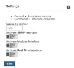
Interface Activation is where SNMP, Modbus, and Real Time TCP Interfaces can be activated. Upon activation, settings for these will appear in the above menu. Multiple interfaces can be active at one time. All interfaces require the DHCP to set to a static IP address.
