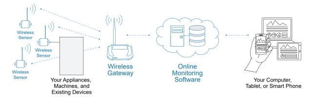
The Monnit solution consists of wireless sensors, gateways and monitoring software, to offer a complete remote monitoring solution. Wireless sensors can be used to monitor various environmental aspects of your business as well as integrate with your existing equipment (such as coolers and appliances) to give you real-time data.
